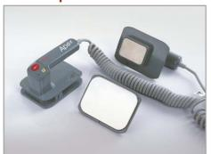
Quickly converted from adult to pediatric by removing the outer surface.
