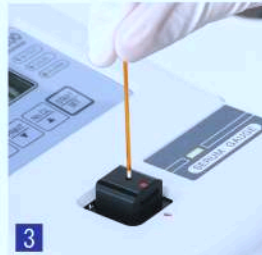
3 Insert a capillary tube (containing a sample) into the holder.
