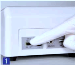
1 Turn on the switch on the rear panel.
