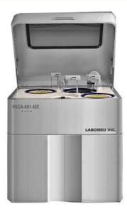
Laborned introduces an automatic biochemistry analyzer with varying testing capacities. FACA-601-ISE conducts 760 tests/hr with True Random Access (600 chemistry tests + 160 ISE).
