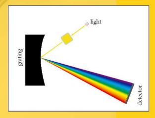
■ High resolution concave grating system, wavelength range 340-800nm, multi-wavelength polychromatic assay at the same time.
