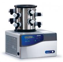
Weight: 102.0 lbs Weight metric: 46.0 kg **Dimensions:** 18.6" w x 18.5" d x 22.5" h Dimensions metric: 47.2 cm w x 47.0 cm d x 57.2 cm h Electrical: 230 volts, 60 Hz, 7 A Collector Temperature: -50°C, -58°F Conformance: CAN/CSA C22.2, UL **Electrical Standard:** Domestic Ice Holding Capacity: 4.5 L **Options Included:** Built-in 10-port Drying Chamber **Plug Type:** North America, 230 volt Style: Benchtop Vacuum Pump Displacement Required: 86 L/Min. or larger displacement
