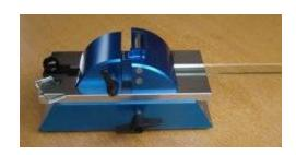
quality glass strips. This glass knife maker will automatically compensate for changes in thickness of the glass strips (typically 5.8 mm to 6.2 mm thick).
