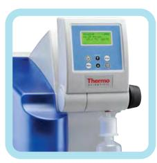
Dispense water which allows for drop by drop or quick dispensing
