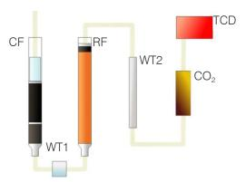
CF = Combustion Reactor WT1 = Water Trap (Physical) RF = Reduction Reactor WT2 = Water Trap (Chemical)  $CO_2 = CO_2$  Auto-regenerating Traps TCD = Thermal Conductivity Detector
