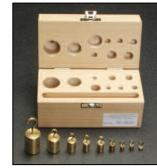
These NEWTON style calibration weights are precision weights use to calibrate force transducers. The weights are made from polished brass and have an integral hook. They are supplied in a wooden storage case. They are calibrated in Newtons at the standard acceleration of gravity gn = 9.80665 m/s2. Nine weights are supplied. Class of accuracy M1.
