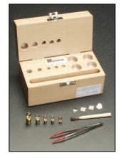
These gram calibration weights are precision weights use to calibrate preload on force transducers. The weights are made from polished brass. They are supplied in a wooden storage case with a pair of handling forceps and a cleaning brush. Nine weights are supplied. The 0.1, 0.2 and 0.5 gram size weights are flat metal pieces. The larger size weights have an integral hook. Class of accuracy M1 after OIML\*.
