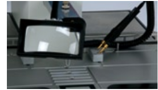
Detail with magnifier and heated forceps
