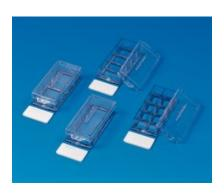
This system features removable, polystyrene chambers that are sealed to a 25x75mm non-fluorescent glass slide using biocompatible acrylic adhesive. The sealant remains with the media chamber after detachment, leaving a hydrophobic border to define cell culture areas. A tabbed cover fits over the media chamber allowing gas exchange while minimizing evaporation. The slides are provided sterile with an RS wash to create a consistent growth surface for adherent cell lines.
