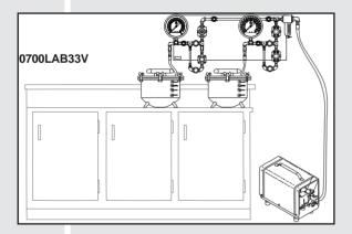
The Model 0700LAB033V# is a multiple porous plate extraction system for laboratory use. This is the extraction system for those that are working in optimum plant water retention values of 5 Bars or less and need extra capacity. Since most water retention studies revolve around optimum plant growth conditions with matric suctions of 5 Bars or less it seems only proper to have a system capacity to handle a number of soils and conditions of most interest.
