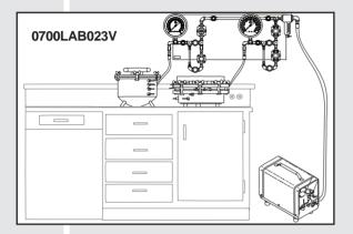
The Model 0700LAB023V# is a multiple porous plate extraction system for laboratory use. This is our most popular lab system providing capabilities for a variety of soils and conditions. The 1500 and 1600 extractors together provide ample flexibility and capacity for low or high water content extraction routines. The combination provides for 2 extractor units for optimum plant growth studies (0-5 Bar Water Retention Studies) while having 15 Bar capabilities as
