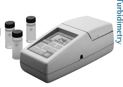
The Hach 2100P and 2100P IS Portable Turbidimeters bring laboratory-level performance on-site, offering fast, accurate results and the ease-of-use analysts demand in the field. With a measurement range of 0 to 1000 NTU and a resolution of 0.01 NTU, the 2100P turbidimeter is ideal for regulatory monitoring, process control or field studies.
