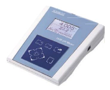
A fully specified laboratory pH/mV/temperature meter that includes full support for good laboratory practices (GLP). The meter supports 1, 2 or 3 point pH calibration on either manually entered pH buffer values or automatically temperature compensated buffers to DIN 19 266, JIS Z 8802 and NIST. Powerful data logging capabilities are included with the ability to store up to 500 readings either manually, at timed intervals or on alarm events.
