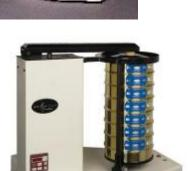
The DuraTap™ Sieve Shaker is a heavy-duty shaker designed to accommodate 8" and 200 mm or 12" and 300 mm diameter test sieves. The tower and wear parts are engineered and constructed with industrial-strength components to withstand everyday, harsh duty cycles. Greased fittings are provided to ensure longer life of the bearings. The built-in digital timer allows for repeatable results.
