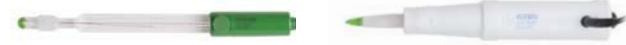
HI10480 PTFE reference, double junction, Clogging Prevention System (CPS), glass body pH electrode with temperature sensor Recommended for wine analysis and solutions with a high concentration of suspended solids
