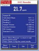
the HI 4222 and HI 4522, the meter calculates the sample concentration automatically and then logs it into an ISE methods report. 200 reports can be saved for future recall. The entire process can be repeated on multiple samples without reentering sets of parameters.
