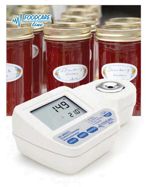
HANNA offers the HI 96821 digital sodium chloride refractometer to meet the requirements of the food industry. This optical instrument employs the measurement of the refractive index to determine sodium chloride concentration in aqueous solutions used in food preparation. It is not intended for sea water salinity measurements.
