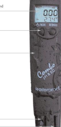
Replaceable pH electrode cartridge
