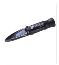
MASTER-2PM are mid-range (measurement range Brix 28.0 to 62.0%) model of the MASTER-M / MASTER-PM. MASTER-2PM are the successor model to the conventional N-2E. The MASTER-M series is a good alternative choice when the water resistant feature is not a priority and the Temperature Compensation will be carried out manually. Not equipped with the Automatic Temperature Compensation feature.
