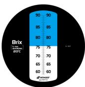
MASTER-3PM are high-range model (measurement range Brix 58.0 to 90.0%) of the MASTER-M / MASTER-PM.MASTER-3PM are the successor model to the conventional N-3E. The MASTER-M / PM series is a good alternative choice when the water resistant feature is not a priority and the Temperature Compensation will be carried out manually. Not equipped with the Automatic Temperature Compensation feature.
