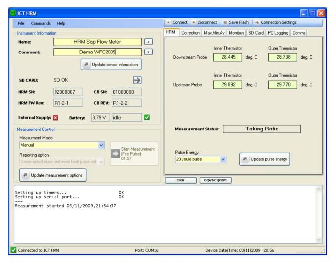
All aspects of the instruments operation and calculations are controlled by the microprocessor which automatically converts the analogue microvolt signals to a calibrated output. Programming variables such as heat pulse interval, energy input, probe spacing's, and measurement frequency are all held resident in nonvolatile memory.
