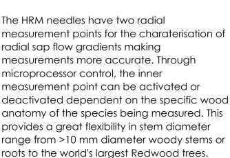
This enables water flows to be monitored in stems and roots of a wide range of different species, sizes and environmental conditions including, drought or water stress.
