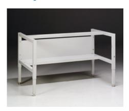
Telescoping Base Stand for use with Purifier® Class II Biosafety Cabinets manufactured since 2000 including the Purifier Delta®, Logic®, Cell Logic®, Logic®+, & Cell Logic®+. Rugged powder coated tube and steel construction. The stand can be installed to provide work surface heights between 30" and 37", in 1" increments. Comes complete with leveling feet and shelf.
