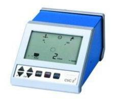
Fully electronic vacuum gauge and controller (two set point control) for absolute pressure determination with built-in piezoresistive pressure transducter (975 - 1 Torr / 1300 - 1mbar) and continuous variable independent setting of two switch points between 106 and 1 mbar (~795-1Torr). Combined analogue and digital read out provided quick and precise information.
